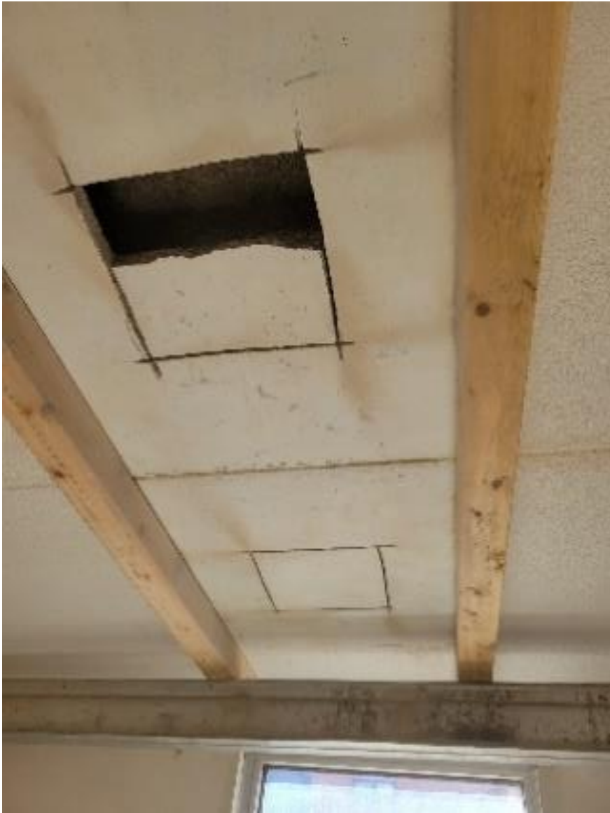
Examples of passing tests – underside of panel stays attached at “web”
